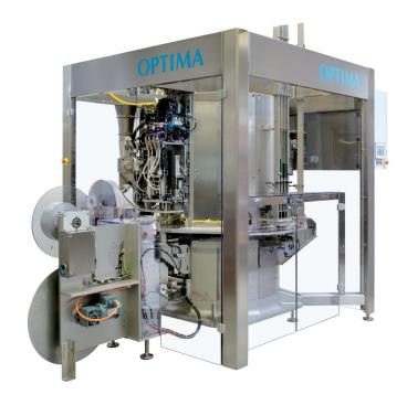
Fig. 2: In contrast to hard pod coffee capsules, HERMES NutriCaps products consist of very fine powders and mixtures of ingredients with different characteristics. Thus, to fill ingredients into the capsules homogeneously and precisely so that content uniformity is ensured and specification limits met, the dosing unit of the OPTIMA CFR 2-2 capsule filler rotary machine was specially modified. (Photo® OPTIMA consumer GmbH)
