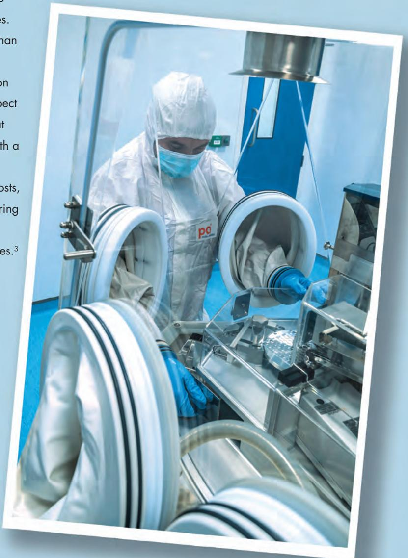
**Often-complex molecules require specialist handling to ensure protection of both operators and the environment (PCI).**
