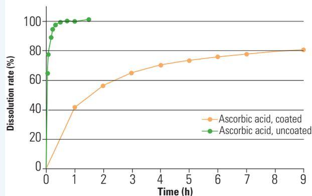
Note: Hot-melt coating was used to create the extended-release characteristics. Dissolution testing was performed using the USP II (paddle) apparatus at 75 rpm, 37 °C, and in 900 milliliters of demineralized water.
