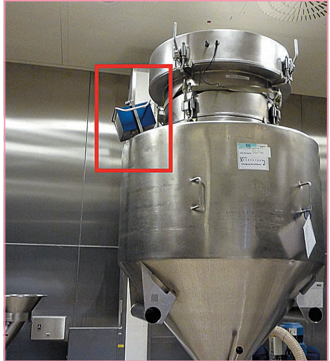
Figure 1: Near infrared spectrometer attached to a production scale blending container. The spectrometer wirelessly transmits data for real-time analysis.
