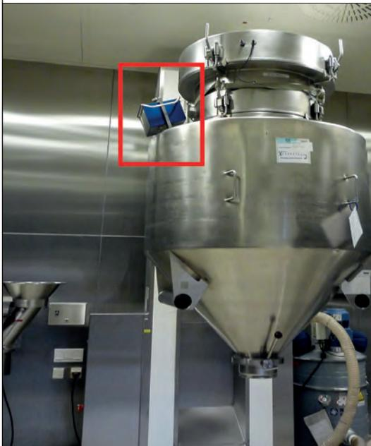
**Figure 3:** NIR instrument attached to a fluid-bed coater: deposits on the NIR probe itself can occur during the coating process but are mathematically corrected for during data acquisition; therefore, the progress of the coating process can be monitored and actively controlled in real-time
