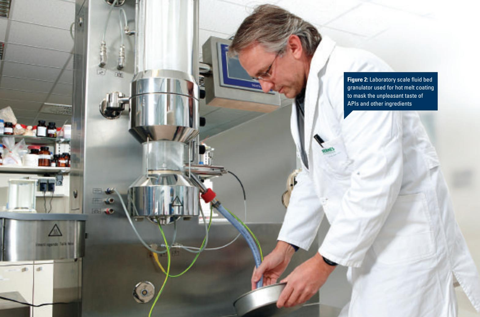
**Figure 2:** Laboratory scale fluid bed granulator used for hot melt coating to mask the unpleasant taste of APIs and other ingredients
